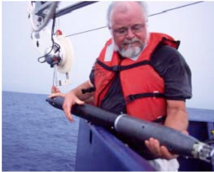
Figure 1. The fast CTD being deployed from the RV REVELLE. The System packages a SeaBird SBE 49 CTD and a micro conductivity probe in a ~30Kg package suspended from a spectra cable with six imbedded electrical conductors. The system is profiled by a portable electric winch at vertical speeds approaching 12 kts.
