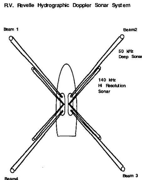
Fig. 1. A plan view schematic of the Hydrographic Doppler Sonar System on the RV Revelle. All sonar beams are oriented downward, thirty degrees off vertical.
