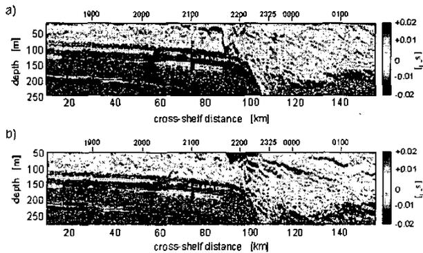
Fig. 4. Shear transects across the Kuroshio in the East China Sea, as seen by the 140 kHz sonar on April 17, 2000.
