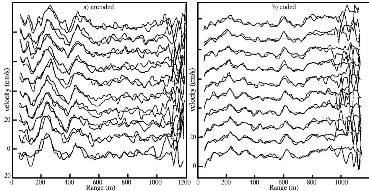
**Figure 3.** A comparison of (a) uncoded and (b) coded pulse performance. Velocity profiles estimated from the 71.5 kHz and 75 kHz systems are overlotted. The disparity between profiles is greatly reduced through coding.
