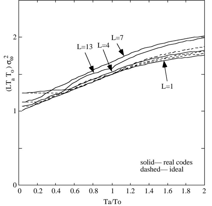
**Figure 2.** Performance of Barker Codes vs. equivalent ideal (pulse train) codes:  $\sigma_{\omega}^2$  normalized by  $LT_{\text{ave}} T_{\text{ovl}}$ . Sequences are 2 13-bit, 4 7-bit, and 7 4-bit subcodes. In practice  $T_{\text{ave}}$  should be set equal to  $T_{\text{ovl}}$ .
