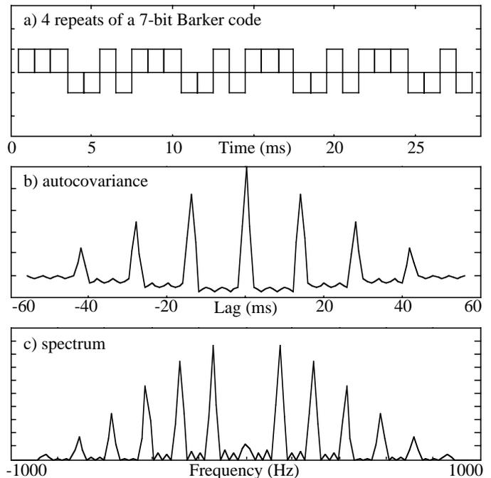
**Figure 1.** a) Schematic Representation of a repeat sequence code. The transmitted waveform consists of a seven bit Barker code repeated four times. b) The corresponding autocorrelation function. Values are small except at even multiples of the subcode length. c) The frequency spectrum of the code. The spectrum of an uncoded sinusoidal pulse of the same duration would consist of a single peak of width equal to the width of any individual peak in the above spectrum.
