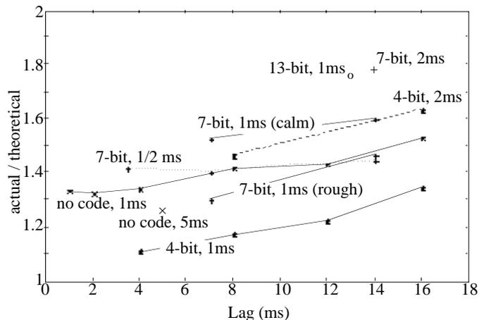
**Figure 8.** Ratios of measured performances to predictions from the theory. Only May 1988 data are plotted, showing a variety of bandwidths and code lengths. The "x" plotted at lag 5, 1.25 ratio corresponds to the uncoded results, interpolated to lag-5 and compared to the theory for data sampled every 5 ms (see text). An overall trend is seen with lag, but a larger variation occurs from code to code. The considerable scatter independent of lag indicates that another parameter is important.
