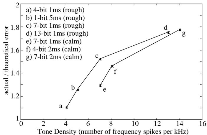
**Figure 9.** Performance ratios vs. "Tone density," or the number of peaks in the code's spectrum per kHz of available bandwidth. The two curves are for the "rough" conditions (upper curve) and "calm" (lower). Note that the uncoded case is plotted according to its (filtered) bandwidth of 200Hz, using the interpolated "lag 5" value. A simple pattern emerges which is apparently dependent on conditions. A simple explanation has not yet emerged.
