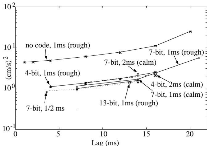
**Figure 5.** Mean-square velocity difference from the May 1988 data, for various codes and lags. Run parameters are noted in the figure; for example, "7-bit, 1ms" refers to a run with 1ms bit-length, repeating a 7-bit Barker code enough times to approximate 28ms total (4 repeats).
