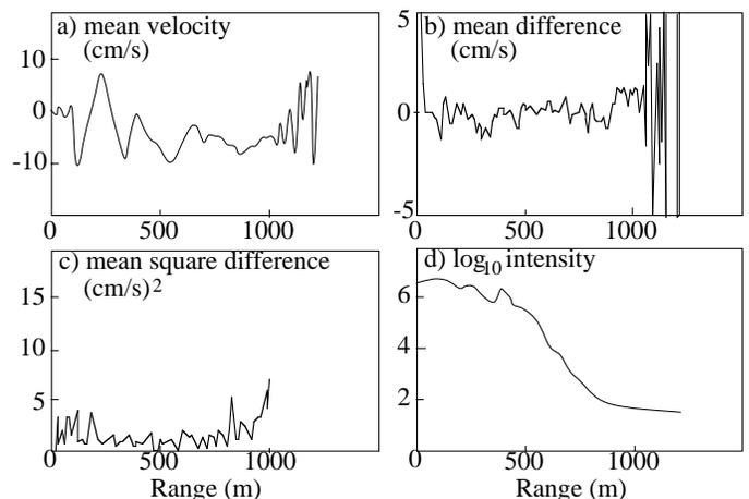
**Figure 4.** (a) The ten minute mean velocity profile, as estimated by averaging results from both the 71.5 and 75kHz sonars. (b) The difference in the ten minute means of individual sonars. (c) The variance of the difference velocity as estimated from 10 one minute profile pairs. (d) The ten minute average acoustic intensity. Variations in the first 200m are obscured by clipping in the A/D converters of the data recording computer.
