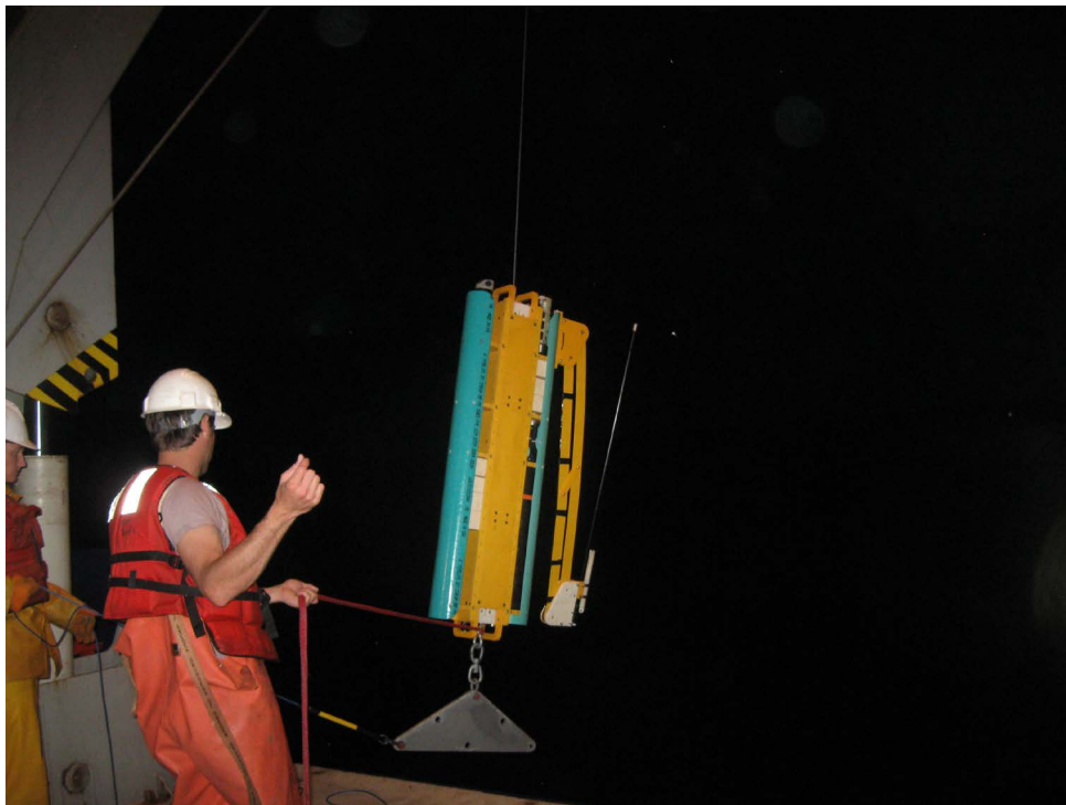
Figure 2. A Macro WW going over the side for a ballasting test. The triangular weights on the bottom of the deployment wire proved too small to keep the wire vertical in the strong equatorial shears. The Macro WWs on the Snake array began to profile well on Dec 24, when the deployment weights were augmented by lengths of chain.
