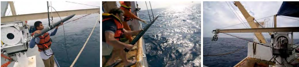
**Figure 2: FastCTD redesigned with a swivelling bale, boom, and powered sheave. The bale allows the FastCTD to collect data during up and down casts. (Photos: T. Hughen)**
